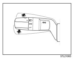
With the headlights on, push the lever forward to switch to the high beams (main beams) or pull the lever toward you to switch to the low beams. When the high beams (main beams) are on, a light on the instrument panel will come on. To momentarily activate the high beams (main beams) as a passing signal, pull the lever slightly toward you and release it when you have completed the signal. Automatic Lights Operation (if equipped)
